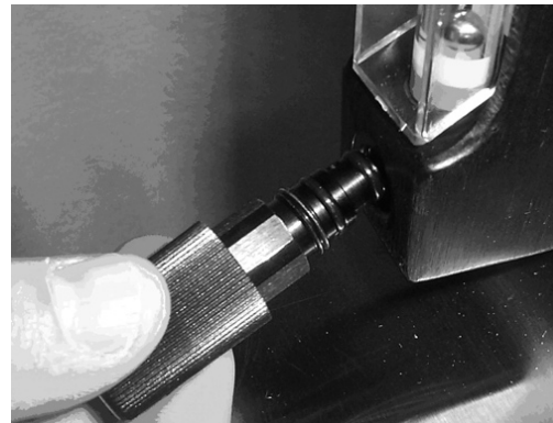
Figure 4-21: Remove Old Needle Valve Assembly
