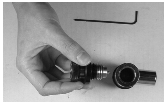
Figure 4-3: Unscrew Assembly from Body
