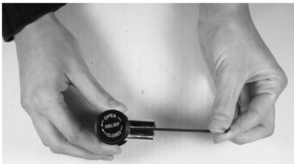
Figure 4-2: Loosen Set Screw on Pop-Off Valve
