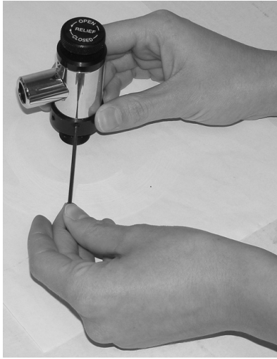
Figure 4-5: Loosen Set Screws
