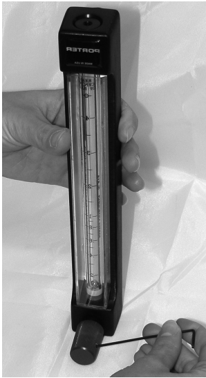
Figure 4-16: Loosen Set Screws in Knob
