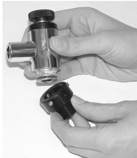
Figure 4-6: Remove Chrome Body from Black Base
