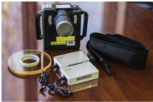
The Image-Vet FleXX™ requires NO installation or assembly. Its two rechargeable batteries, neck strap and back scatter shield all fit conveniently in the supplied hard-shelled transport case (not pictured).
