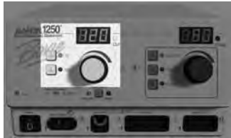
Figure 2 – 2 Controls for the Cut and Blend Modes
