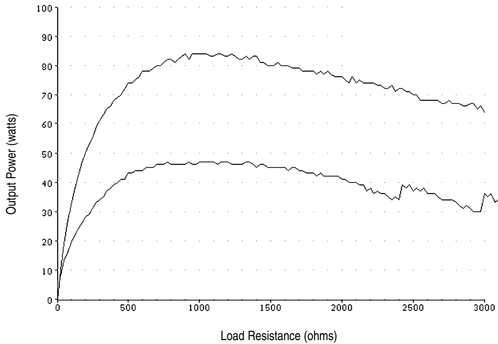
Figure A - 5 Output power versus impedance for Coagulation mode
