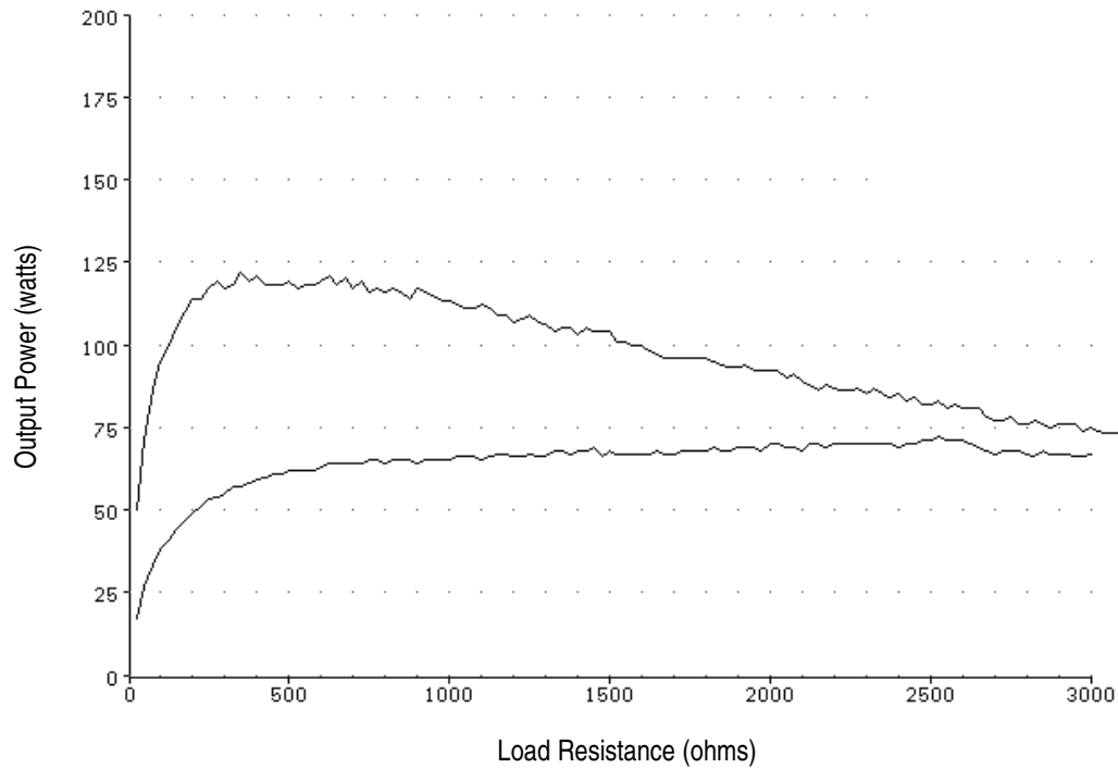
Figure A - 1 Output power versus impedance for Cut mode
