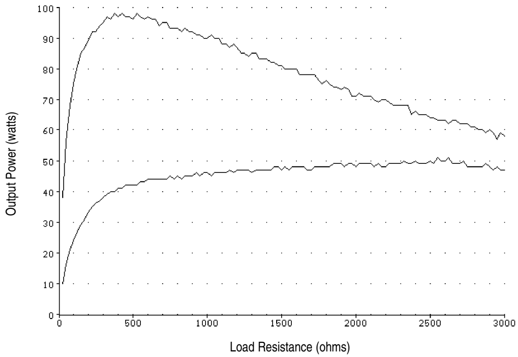
Figure A - 3 Output power versus impedance for Blend mode
