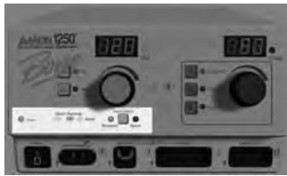
Figure 2 – 4 Indicators for power, return electrodes, and footswitch control
