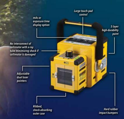
High output, low weight and hundreds of exposures from a single battery charge, packaged in one of MinXray's most durable designs – the **TR90B Tough Ray Battery Powered** portable x-ray unit. Compact but powerful, field tested and field ready, features of the **TR90B** include:
