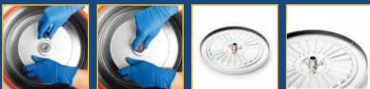
**NOTE:** Please ensure that the black rubber rotor gasket is positioned around the rim of the rotor such that the capillary tubes are pushing into the rubber while spinning. The rubber gasket is not affixed to the rotor to allow for cleaning and re-positioning of the gasket to prolong gasket life.
