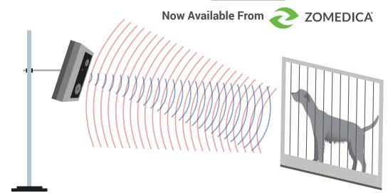
VetGuardian<sup>®</sup> monitors pulse and respiration based on patented Continuous Waveform Doppler RADAR technology.
