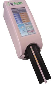
The InSight Urinalysis reader is a semiautomated urine test strip reader with touch screen and printer to be used in conjunction with InSight Urine Test Strips. Dip the strip into the urine and place it on the strip loader ....have your results in 60 seconds.
